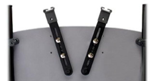
Shoulder Harness Guides Installed
